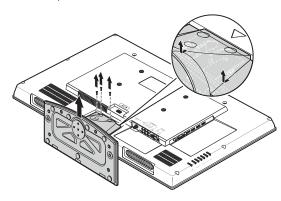
3 Secure the wall mount bracket to the back of your TV using the four screws provided with the bracket.
